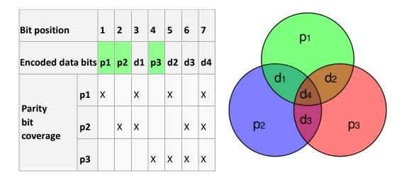
Here, d1, d2, d3, d4 are the 4-bit data and p1, p2, p3 are the parity bits. From this table it is obvious that parity bit p1 is calculated from data bits d1, d2 and d4 and all data bits are covered by at least 2 parity bits.
