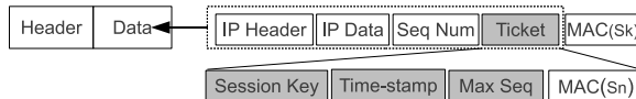
Fig. 2. MON packet structure. User’s IP traffic is encapsulated into a new transport layer packet to enable routing by MON nodes, including an encrypted access ticket and message authentication code to ensure MONs’ message integrity, and authenticity. Only entry nodes can decrypt and validate the ticket.
